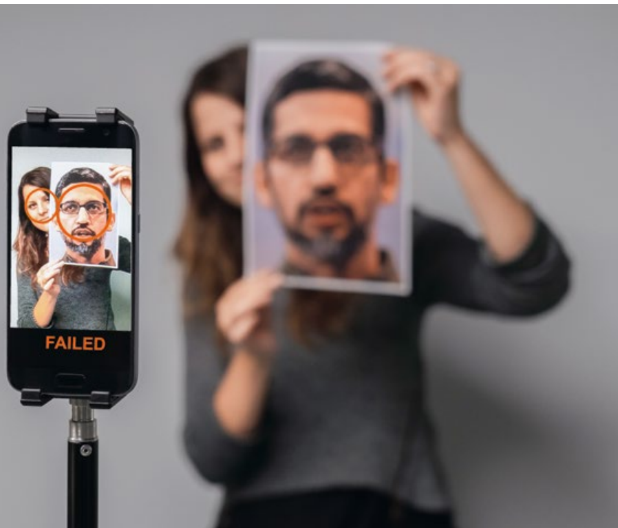
← The so-called presentation attack consists of trying to fool a facial recognition system by presenting a photo (or a mask) instead of the user’s face. Here, Idiap uses a photograph of Sundar Pichai, Google’s CEO, to test Android’s facial recognition system.
